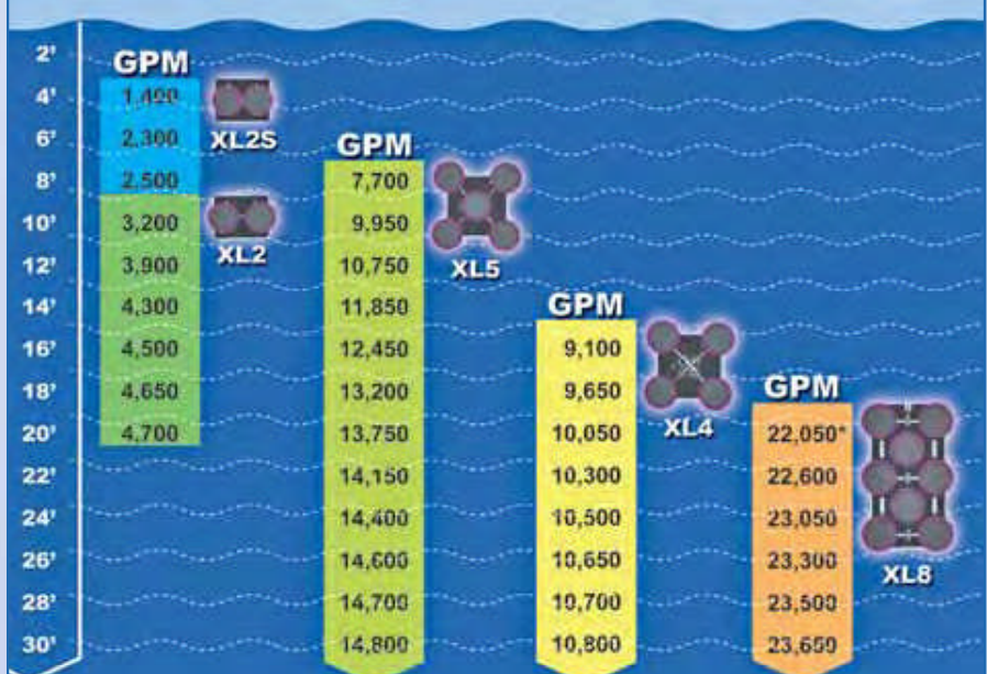
Vertex Diffuser Models Categorized by Lifting Rate GPM (Gallons Per Minute) and Water Depth Air flow = 1.0 CFM (Cubic Feet Per Minute) per disk
